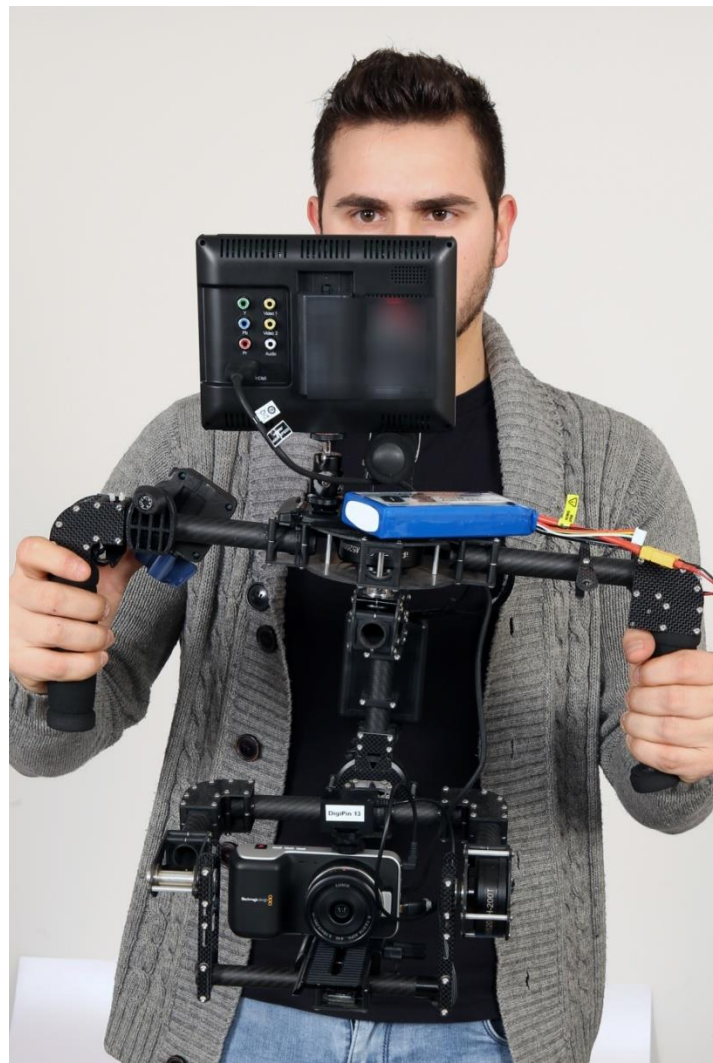
WL2 mounted on a Gimbal (front view):
