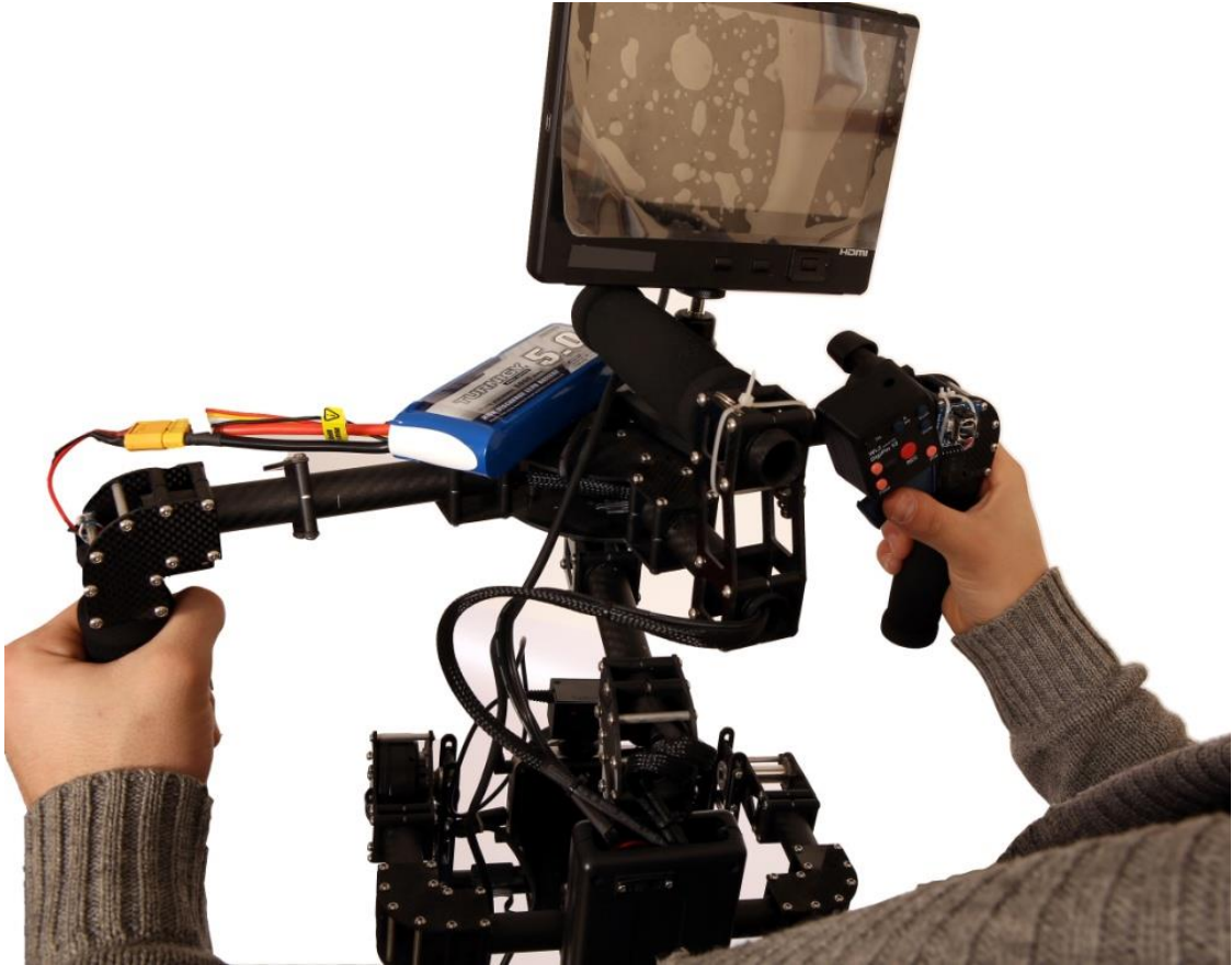
WL2 mounted on a Gimbal (Rear View):
